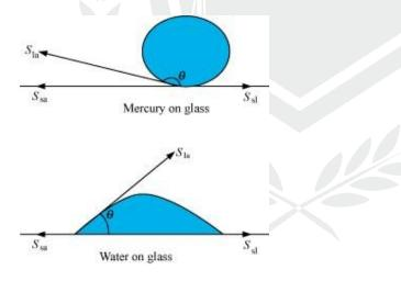
$S_{la}$ ,  $S_{sa}$ , and  $S_{sl}$  are the respective interfacial tensions between the liquid-air, solid-air, and solid-liquid interfaces. At the line of contact, the surface forces between the three media must be in equilibrium, i.e.,
