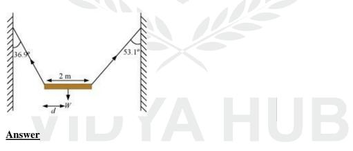
The free body diagram of the bar is shown in the following figure.
